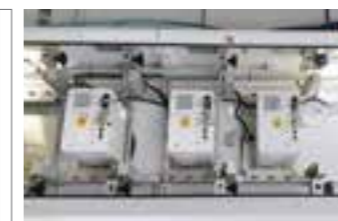
Simultaneous measurement by several FISCHERSCOPE® X-RAY 5100
