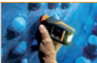
MMS® INSPECTION DFT: Measurements of thick layers
