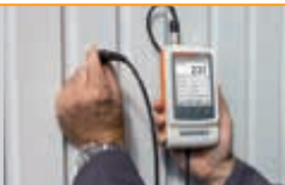
Measuring paint coating on steel
