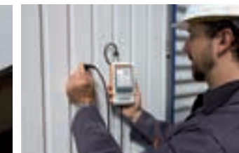
Measurement of a paint coating on steel
