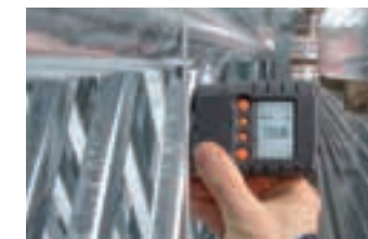
Measurement of anodizing on aluminum frames for building cladding
